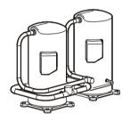
**Capacity control.** The FM modules utilize tandem scroll compressors for two-step modulation. One or both of the compressors can run depending on the load of the system. This feature allows for up to six steps of "true" unloading in a three-module system without the power factor and friction penalty of an unloaded semi-hermetic compressor.
